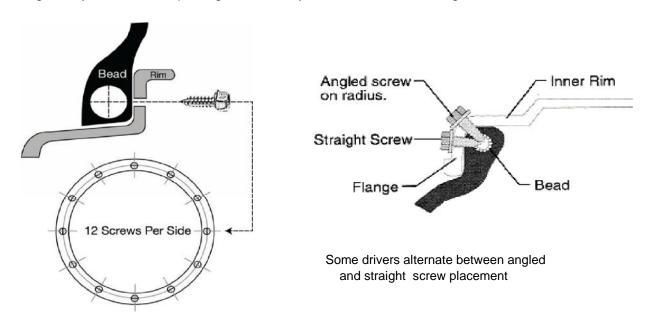
Do NOT: Never drill any holes with the tyre still fitted to the rim
